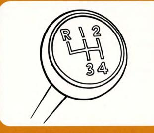
Volvo's standard transmission has four forward speeds. Change gears as in any other shift car. To get into reverse pull the lever all the way to the left to get past the detent (you'll hear a click), then forward.
