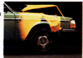
Crumple zones front and rear absorb as much energy as possible in the event of a collision.
