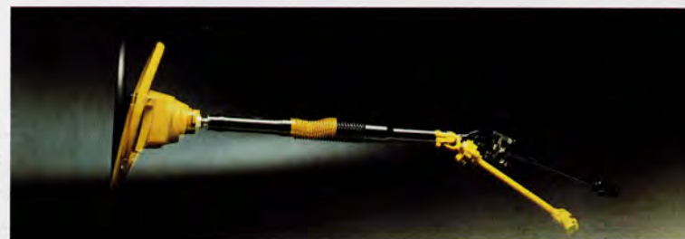
The collapsible steering column is designed to offer several stages of protection to help minimize injury.
