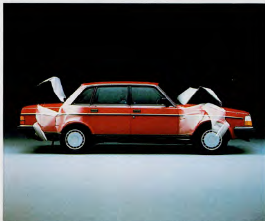
Front and rear body sections are designed to help absorb impact forces by crumpling in a predetermined manner.
