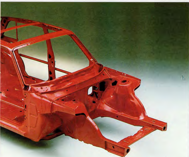
In unitized construction the frame and body shell are designed as an integral unit. The whole body is designed to act as a safety cage to help protect the driver and passengers in the event of a collision.
