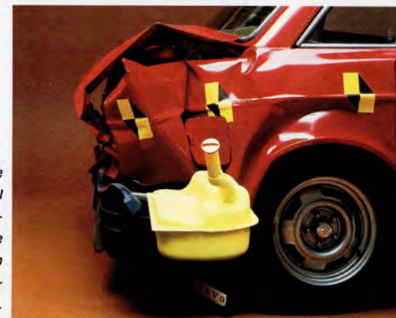
The fuel tank is placed close to the rear axle. The fuel pipe incorporates two bellows-type joints that provide a degree of "give" to help reduce the risk of fuel leakage during an accident.
