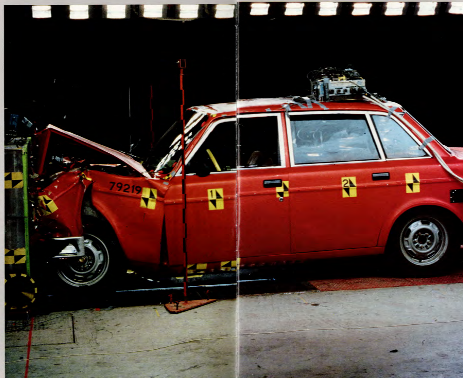
Volvo's unitized body creates a kind of cage that surrounds passengers on all sides.
