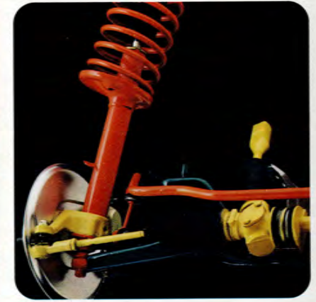
THE FRONT SUSPENSION INCLUDES MCPHERSON STRUTS WHICH INCORPORATE COIL SPRINGS AND SHOCKS.
