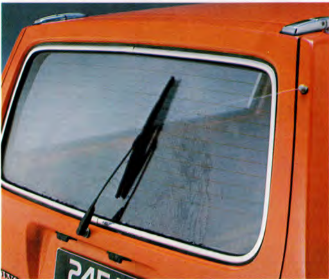
Rear visibility is of great importance. The Volvo 245 Challenger Van is fitted with an electrically heated tailgate window, which is kept clean by a wiper/wash unit.
