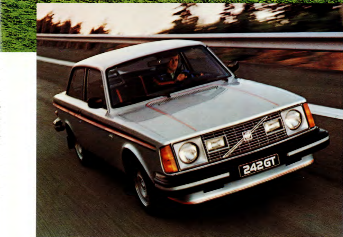
242GT Volvo's 242GT makes a fine road car even better. Higher rate springs, heavy duty shock absorbers and a thicker front stabilizer bar stiffen the GT's suspension for more precise handling. Special interior and exterior trim, a GT steering wheel, Pirelli high performance radials and light-alloy wheels are just some of the standard features. The 242GT engine is the same spirited four with C.I. fuel injection and Lambda-sond™ emission found in other 240 Series cars, the same power plant that has raised Volvo performance to the level expected and demanded by motoring enthusiasts.
