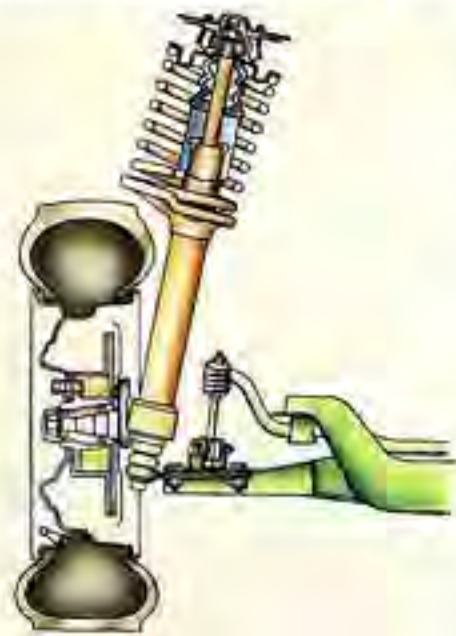
Cross-section showing the McPherson strut suspension.
