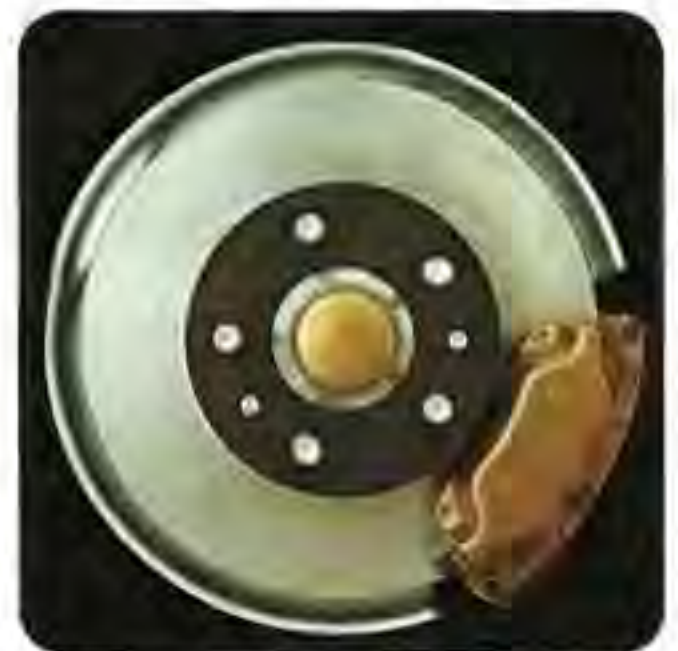
Four-wheel disc brakes are standard. The front discs are ventilated on the 242GT and 260 Series.
