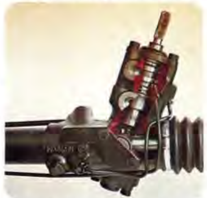
Power-assisted rack-and-pinion steering provides precise, positive control. It is standard on most Volvo models.
