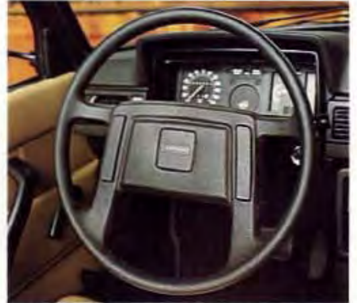
Padded safety steering wheel, variable-intensity illuminated instrumentation.
