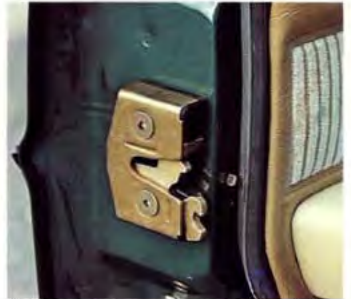
Door latches have built-in drains; water that gets in runs out.
