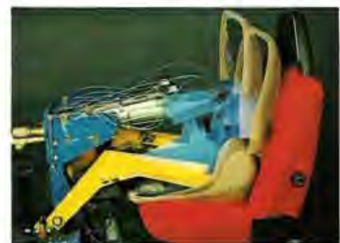
Volvo's reputation for toughness isn't just because of thick paint. Volvo also invests heavily in sophisticated testing and quality-control equipment and procedures. This machine, for instance, can put years of stress and wear on a seat in a matter of days. It represents Volvo's dedication to quality.
