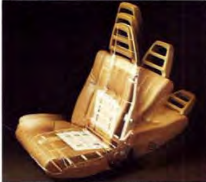
For added comfort in the cold of winter, a heated driver's seat on 260 models.
