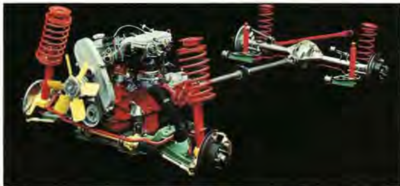
Volvo 240 and 260 Series cars ride on a front suspension with McPherson struts, coil springs, internal shock absorbers, stabilizer bar and rack-and-pinion steering.
