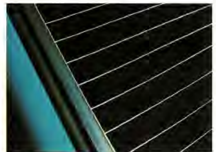
It takes 1292°F to burn the special demisting heating elements into the rear-window glass, and the elements draw 150 watts of power for quick clearing of ice or mist to give the driver an unobstructed view to the rear.
