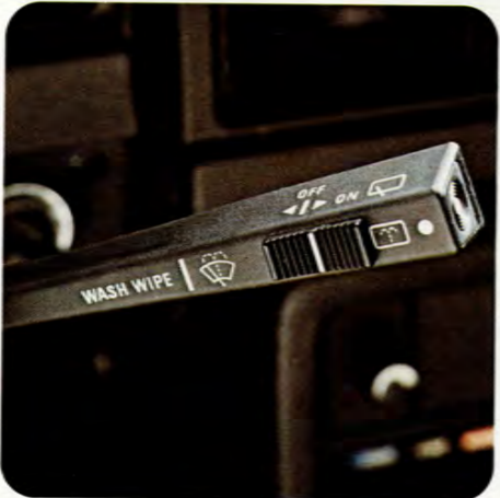
The rear window wiper has an intermittent cycle on the 265GL, which is available for the 245. The control is on the steering column.
