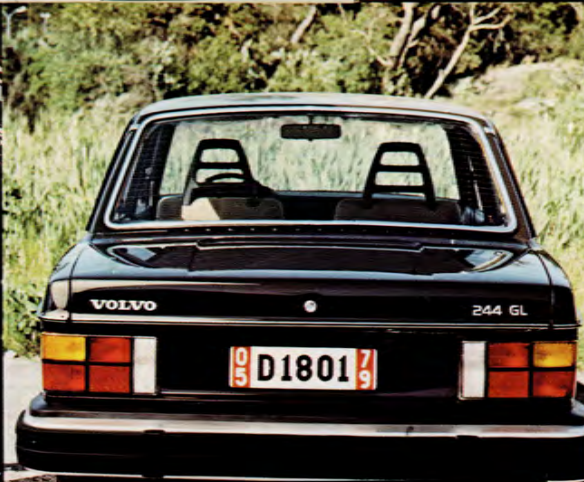
The new boot lid of the 240 series is rounded and smoother in shape. A new barrel lock, which can only be opened with a key, helps prevent theft of luggage.
