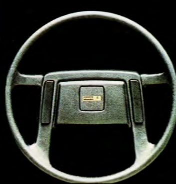
The safety steering wheel incorporates two operating bars for the horn.
