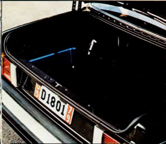
The new design of the Volvo 240 series includes a 90 mm lower boot lid, which makes it easier to load and unload luggage.
