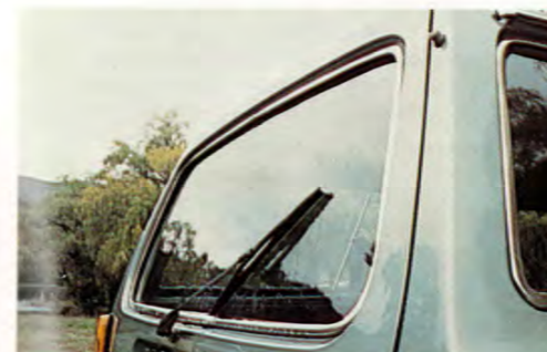
The rear window has heating elements laminated in the glass and its own washer/wiper.
