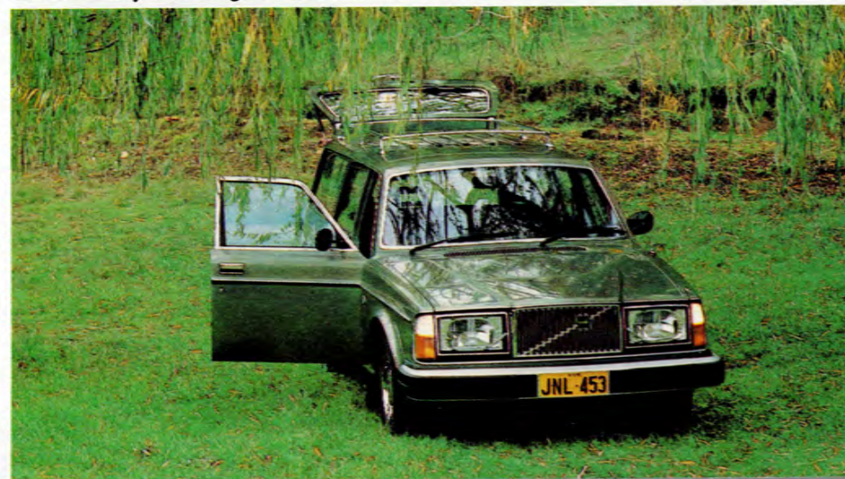
The big cargo area (around 2 cubic metres with the rear seat down) is only 59 cm above the ground, with no awkward threshold to heave loads over. The big door swings up high, right out of the way. The integrated roof-rack shown below comes as standard equipment.
