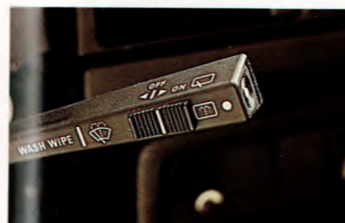
The wiper/washer stalk on the steering wheel column now has a switch for the separate tailgate wiper/washer.
