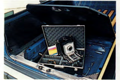
A special 59dm 3 compartment under the floor for concealing valuables when the car is parked.
