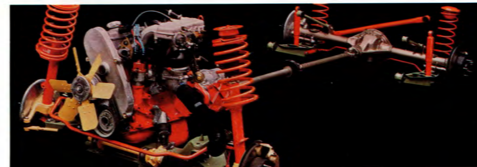
Volvo's outstanding handling is due to a number of factors, like precise rack and pinion steering, spring strut front suspension, a live rear axle with coil springs and an anti-roll bar and ideal weight distribution to make the car well balanced.
