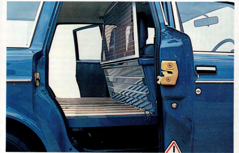
The cargo area is 2 metres long with 2.2m 3 volume. The metal floor with wooden strips is hard wearing and easy to maintain. The large rear opening and side rear doors allow easy loading for the entire cargo area.
