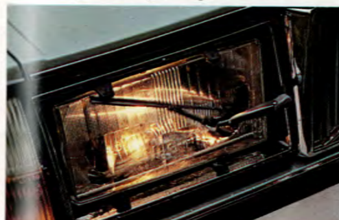
The big halogen headlights have separate high/low beam reflectors and washer/wipers to keep the glass clean.
