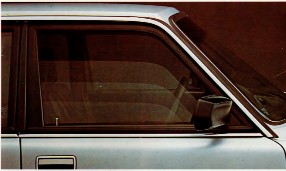
Electric windows, front only on 245GLE/265GL, rear windows too on 265GLE. Controlled from a panel on the driver's arm rest.
