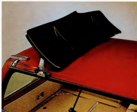
With fuel economy such an important consideration, a roof spoiler is a 'must' when towing a caravan. By improving the aerodynamic line of the rig it reduces wind resistance and can improve fuel economy.
