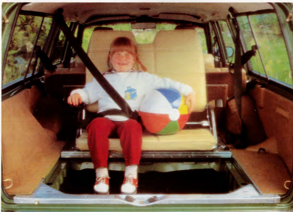
This rearward facing extra rear seat turns your Volvo estate into a seven-seater. Especially suitable for children, it is equipped with head restraints, three point seat belts and armrests. Upholstered in easy-to-clean black or beige vinyl, it folds away under the cargo area floor when not in use.
