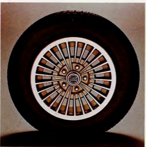
Alloy wheels reduce your car's unsprung weight and increase brake cooling. This 25 spoke 'sunburst' design polished aluminium alloy wheel is available with either a small (as illustrated) or large hub cap.
