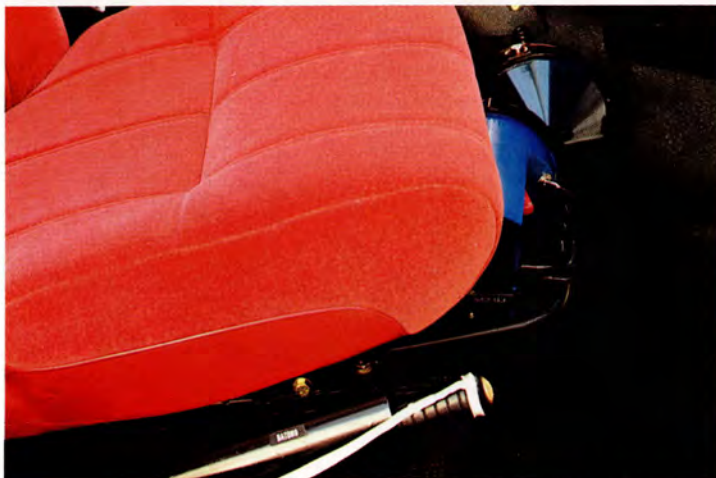
Truncheon holders beside front seats. Holders for hand-held searchlight. Fits under right front seat.
