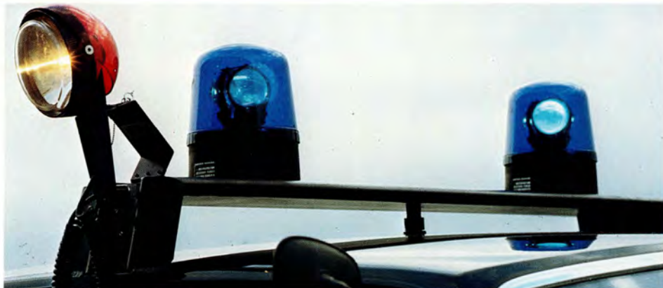
The police lamps can be fitted directly on the roof or on a special roof module. The module includes attachment points for a hand-held, halogen searchlight.
