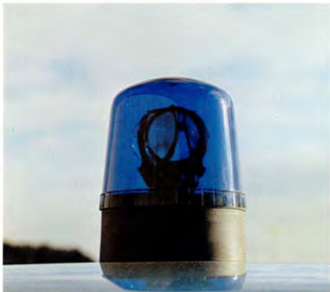
The police lamps can be fitted directly on the roof or on a special roof module. The module includes attachment points for a hand-held, halogen searchlight.
