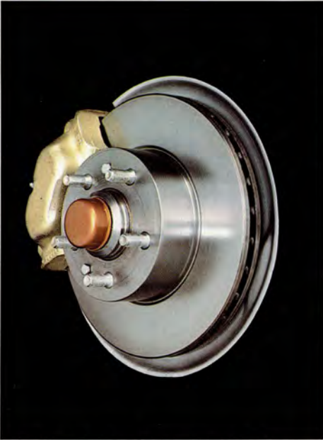
The front disc brakes are ventilated to eliminate fading — even after repeated heavy braking.
