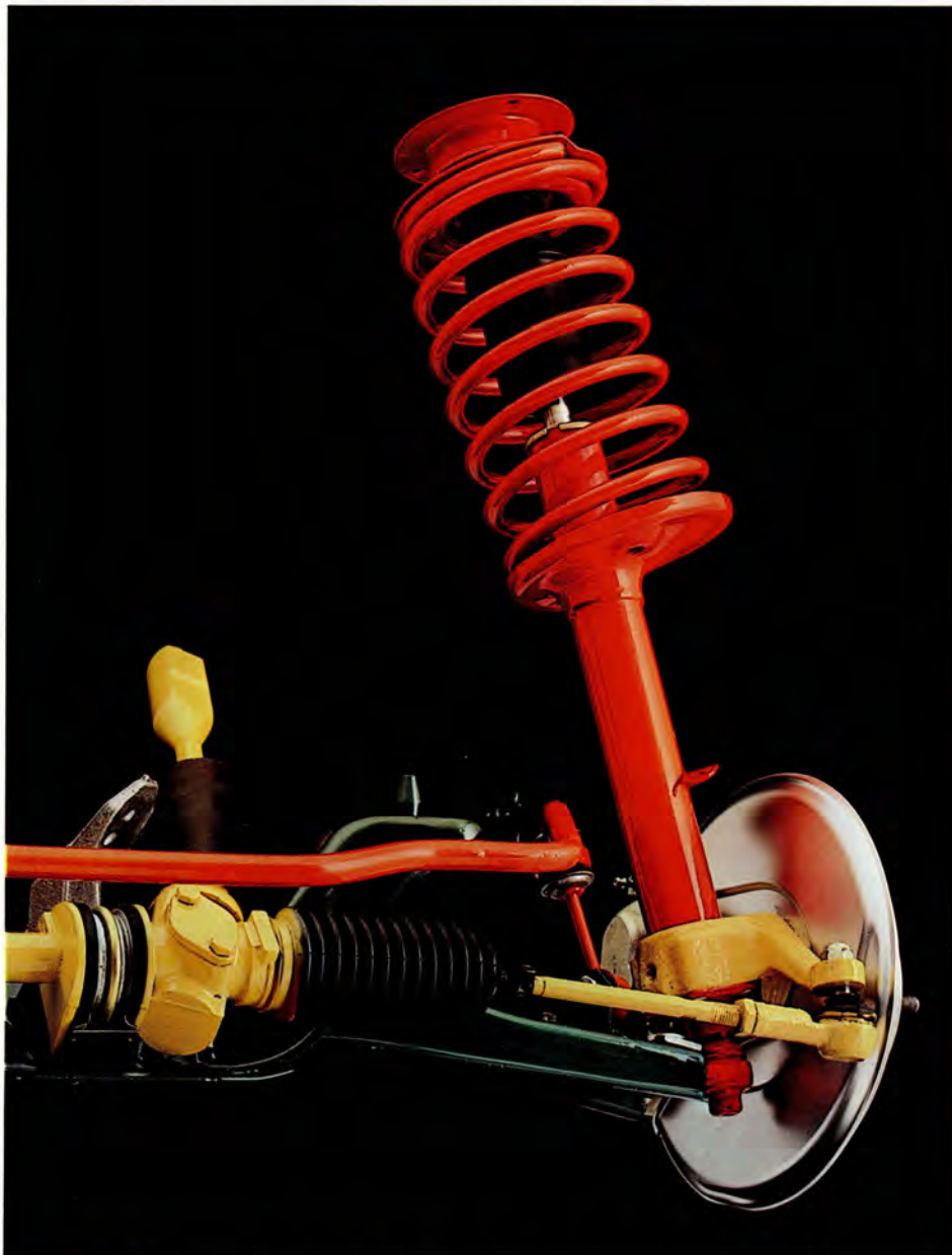
Front wheel suspension with individually acting spring struts provides stable steering characteristics in all situations.
