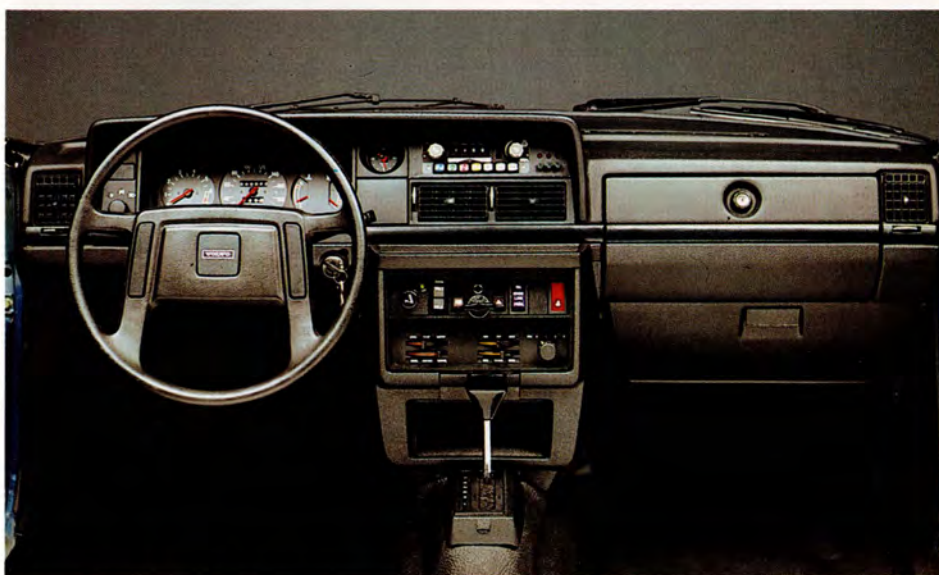
Space in dashboard for two-way radio. The electric equipment can be fully suppressed. An optional compartment can be placed beneath the glove compartment.
