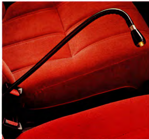
The flexible map reading lamp can also be mounted beneath the dashboard.
