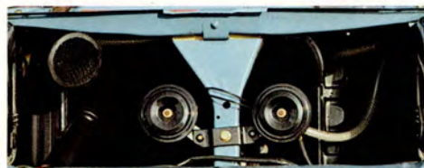
Siren positioning optional. Shown here behind the grille for extra protection.
