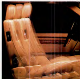
◀ Both front seats offer a "memory" glide feature that allows easier access to the rear seat.
