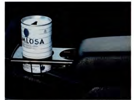
Armrest with Beverage Holder - Convenient sliding tray design provides beverage holders for front and rear passengers. It holds up to four beverages or cups. The elevated armrest enhances driving comfort.
