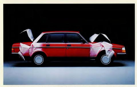
**Safety** Volvo's crash safety system is based on a simple, three-fold approach. Initially, the front and rear designed-in "crumple zones" help to absorb collision forces. Next, the passenger compartment is designed to act as a "safety cage"; and, finally, the three-point seat belts and interior design help form a last line of defense.
