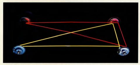
of Volvo's stepped-bore master brake cylinder. To help combat wheel lock-up, the 240 incorporates a special relief valve, to help distribute braking effect equally between front and rear wheel disc brakes when you hit the pedal hard.
