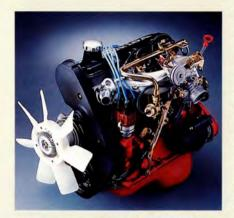
Engine The 240 Series Volvos feature our in-line, four-cylinder B230F gasoline engine, with single overhead camshaft, electronic ignition system with spark advance and knock sensor, LH-Jetronic fuel injection, and Lambda Sond\* emission control. It's a low-friction power plant with a highly efficient lubrication system, lightweight pistons, and a precisely balanced crankshaft.
