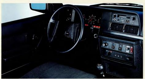
"User-friendly" best describes the 240's instrument console. With a cover angled to reduce glare, adjustable panel lights, and controls located within easy reach, you can command your sedan safely and in comfort.
