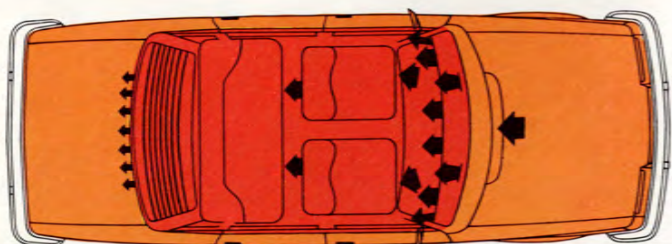
The new Volvo 264 GL has a highly efficient heating and ventilation system of the through-flow type designed to cope with extremes of weather. There are four adjustable nozzles on the dashboard which you can set from fully open to tight closed in any direction you want.
