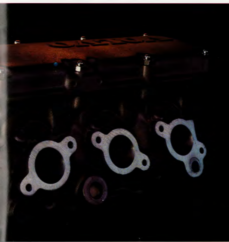
Light-alloy cylinder head features a camshaft over the valves. The intake air/fuel mixture enters from the near side, exhaust gases are released to the far side.
