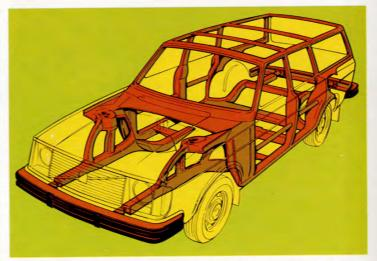
Structural strength and torsional rigidity of the rugged unit-body of Volvo's wagons forms the basis for overall passenger protection, but surrounding the passenger compartment itself is a protective "cage" of closed box-section pillars.
