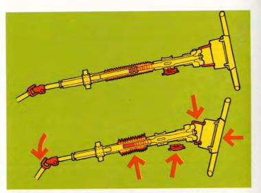
The Volvo steering column offers multiple stages of protection. First there's the padded, deformable wheel housing. Then the steering column, which is designed to collapse in two stages. Finally, a universal joint allows the column to fold like a penknife.
