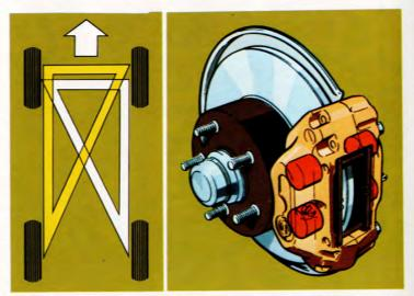
With Volvo's unique triangle-split brake system, both front wheels and one rear wheel are served by two independent circuits. Should one circuit fail, a Volvo will still retain about 80 % of its full braking power. Power disc brakes at each wheel are also standard.
