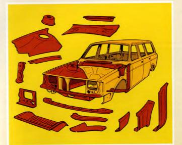
Volvo's are designed to last. Galvanizing and the application of rust proofing fluids and compounds are used extensively on all models. Before a body is finished in enamel, it is etched, electro-dipped in primer, sanded and spray primed.
