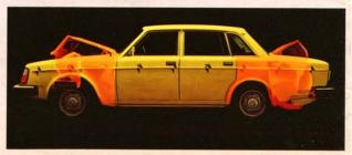
Rigid members of the body form a protective cage around passengers. In addition to pillars and side-guard bars, the floor pan is reinforced by a large traverse box section. Special patterns stamped into the panels of the built-in "crumple zones" allow major impacts to be absorbed at controlled rates.
