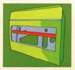
To protect occupants in the event of side impacts Volvo reinforces the doors of every car it makes with tubular pro-
