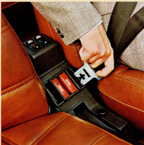
Floor console contains illuminated latches for self-adjusting 3-point safety belts, controls for power rear windows and remote-control outside mirrors.
