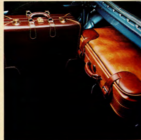
The tall, container-like luggage compartment is proportioned so that suitcases can be stowed vertically.
