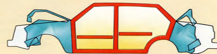
At both ends of Volvo's unitized body are zones designed to absorb impact before they get to the passenger compartment. Parts of the body have been stamped with special patterns allowing them to crumple at a controlled rate.
