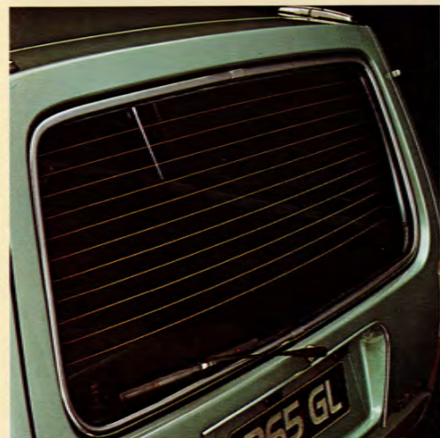
The rear window is equipped with a washer and wiper for rain and road grime and a 150 watt defroster to clear ice or mist in minutes.
