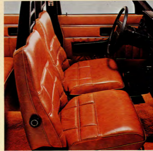
The 265 GL driver can adjust the seat nine ways. It's heated automatically when the temperature drops below 57 degrees.
