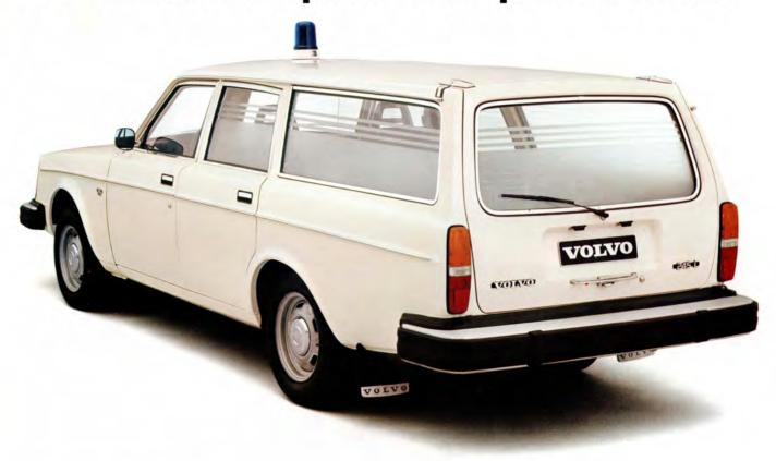
The Volvo 245 Hospital Transport Vehicle is a versatile model designed and equipped for less severe ambulance service. It can also be used as a personnel transporter.
