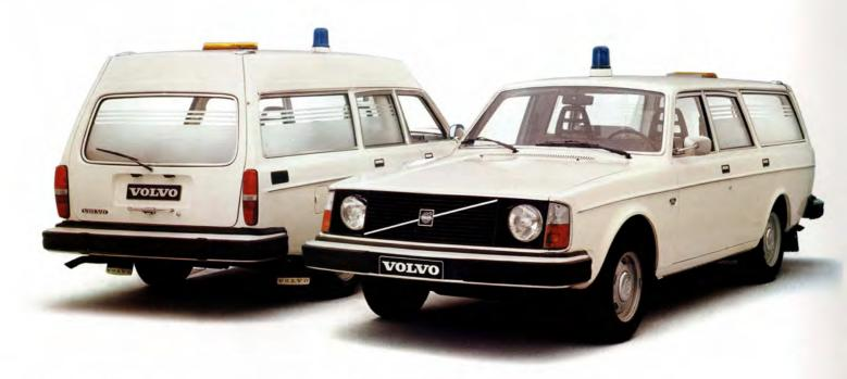
The Volvo 245 Mini-ambulance is available in either standard height or with a lifted roof-line. Both types are powered by a four-cylinder, 100 hp engine with an aluminium alloy cross-flow cylinder head and an overhead camshaft. Utterly reliable, with plenty of power for speedy and safe overtaking.
