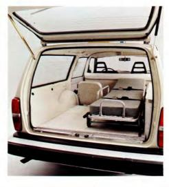
Both versions of the Mini-ambulance are upholstered and trimmed with the same type of attractive, easy-clean materials. Only the roof height above the stretcher differentiates these two models. Standard height in the Miniambulance is 57 cm between the stretcher and roof-lining.
