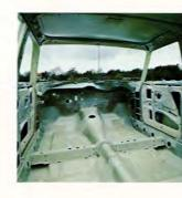
The integral, all-welded steel body has reinforced boxsection profiles around all body openings. Comprehensive rust-proofing and underbody sealing are standard.
