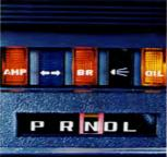
The optional three-speed automatic has a column mounted shift lever and an illuminated quadrant with standard P-R-N-D-L pattern.
