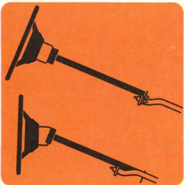
New steering wheel with built-in crumple zone and aligning feature.
