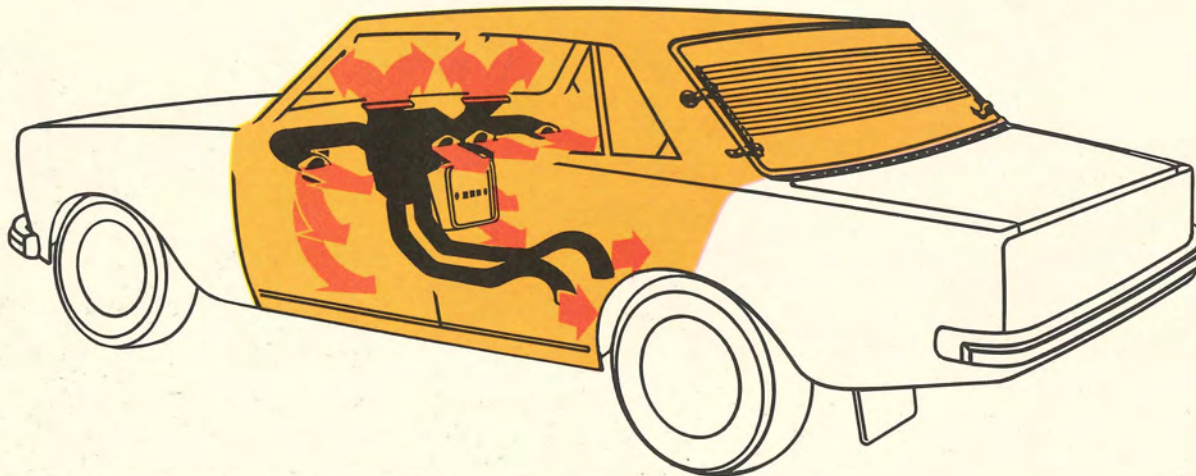
Completely new heating and ventilation system with 10 outlets.
