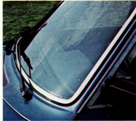
Tinted windshield, three-layer laminated "high-impact" design.
