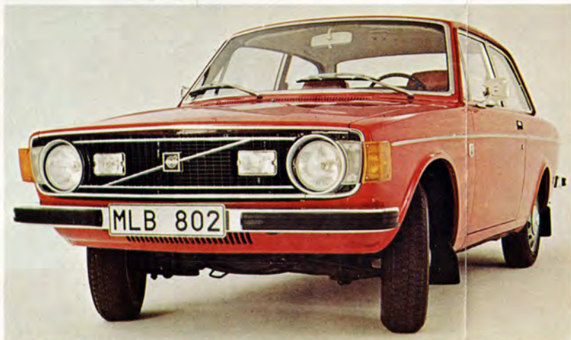
GRILLE LAMP KIT Consists of either two fog or two spot lamps with a special grille section. The quartz iodine lamps are well-protected — reduces risk of theft or damage. 140 series
