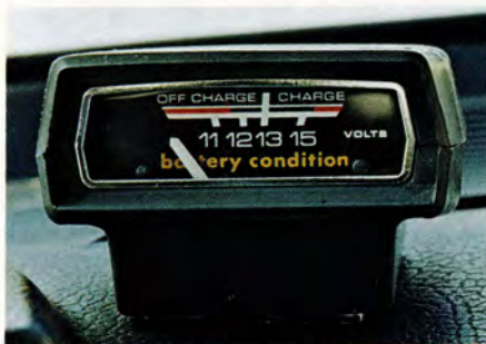
BATTERY CONDITION INDICATOR Provides constant information on the voltage output of your electrical system. If your battery is weak, find out before it fails, particularly during winter.
