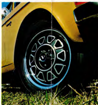
GT WHEEL Exclusive "mag"-type wheels with light alloy centres, steel rims emphasize Volvo GT character, add to performance. Chromed hubs and nuts also available. All models
