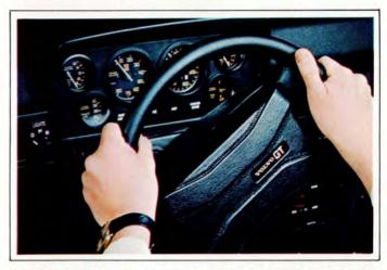
GT STEERING WHEEL — Smaller in diameter than the standard wheel, covered with high quality simulated leather. Fulfills all safety standards. All models
