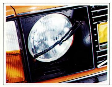
HEADLIGHT WIPER/WASHER—A sensible safety accessory designed to keep your headlights clean in the dirtiest driving conditions. All models
