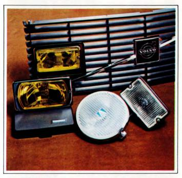
GT AUXILIARY LAMPS — A complete range of fog and driving lamps in bumper-mounted or grille-kit mounted styles is available. All models
