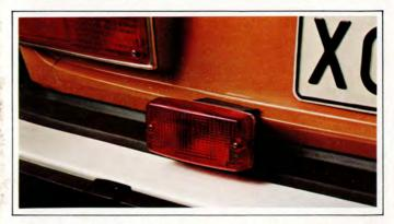
**REAR FOG LIGHT**—A safety necessity when driving in very foggy conditions, this high-intensity red light warns following motorists of your car's location. All models
