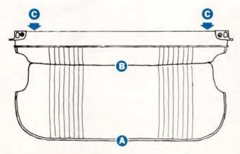
Press the seat cushion down in the front center (A) and then lift the cushion up at (B). The seat cushion will fold forward against the backrest. Then fold the rear seat backrest down by grasping either of the handles (C) on the backrest and folding forward and down.
