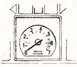
Standard on the 164E and 1800ES, and optional on 140 Series models, the tachometer enables the driver to measure engine speed for better performance, economy and efficiency. Use the gear giving the lowest engine speed for best economy. Best performance is obtained above 3500 rpm. Keep the engine speed below the red line, where horsepower begins to fall off and to avoid overstressing the engine.
