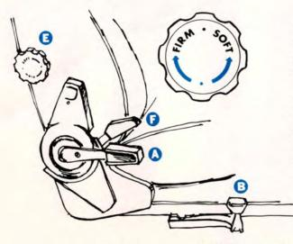
Raise lever A straight up to adjust the backrest from upright to a reclining position, or to any point in between. Then push the lever down to lock the backrest in place.
