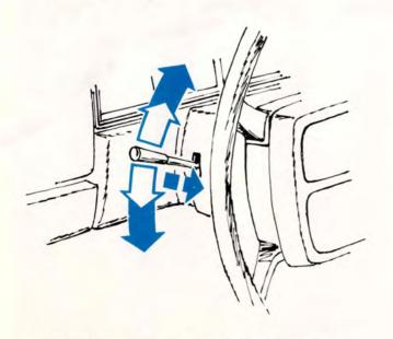
Push the lever *all the way* up or down to indicate a turn. To indicate a change of lane, push the lever *halfway* up or down and hold it until you have moved into the other lane. When you let up on the lever, it will automatically return.
