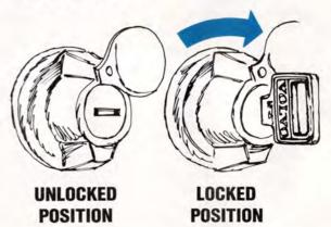
The trunk can be left locked or unlocked if desired. If the trunk is unlocked, it can be opened by turning the knob to the right to release the catch.
