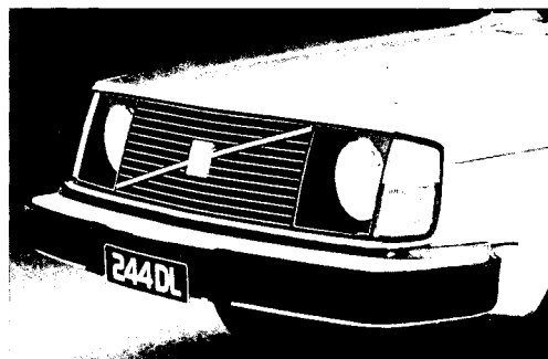
8. Energy absorbing bumpers prevent structural damage to body in 'parking speed' impacts up to 5 k.p.h.
