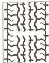
Wear indicator exposed. Tire is worn, replace.
