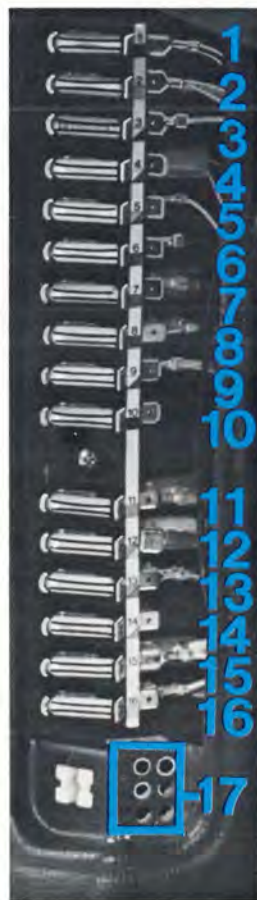
17 Fuse storage, spare
