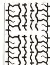
Wear indicator exposed Tire is worn, replace
