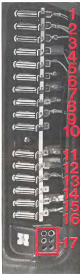
17 Cavity for spare fuses
