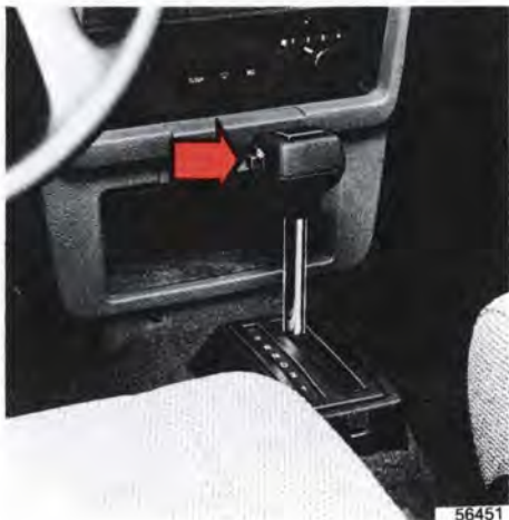
Overdrive indicator light. The light is on when overdrive is disengaged.
