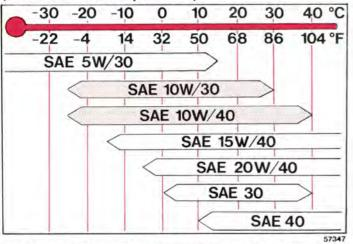
SAE 15 W/40 or SAE 20 W/40 oils are recommended for use in extreme driving conditions that involve excessive oil consumption and high oil temperatures e.g. mountain driving with frequent decelerations or fast motorway driving. (Note however the lower temperature limits.) Capacity: 6.5 litres. Oil-level check: When refuelling
