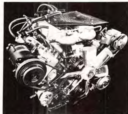
Volvo worked with Renault and Peugeot to develop this new OHC V-6.
