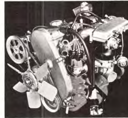
B-21F sohc four; cam is belt-driven.
