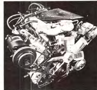
The B-27 2.6-liter V-6 has overhead cams, is all-aluminum and uses Bosch CIS fuel-injection.
