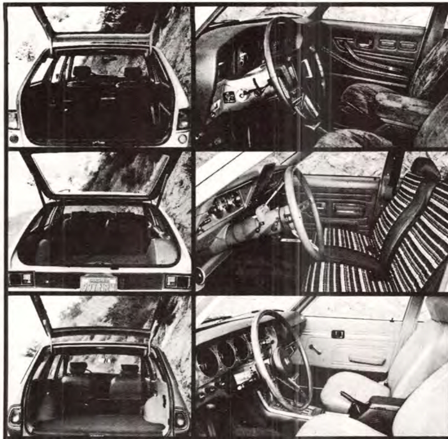
Mazda's cargo area (top) features lockable storage compartments on either side, under-car spare storage. Slide-in access to Hornet's cargo area (center) is hampered by raised end of rear body section. Space Saver spare is housed in covered compartment at right. Like Hornet, the Toyota (bottom) has large wheelwell intrusion that narrows floor width in that area.
