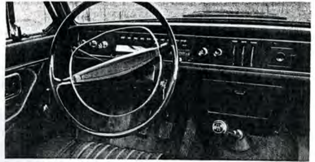
Left: The engine is the well-proved B.18 unit, shown here in "S" tune with twin S.U. carburetors. The cooling system is sealed and all reservoirs are easy to reach and see-through plastic. Above: Interior styling is modern with all-black trim and much crash padding. The long central gear lever is positive to use and there is face level ventilation.
