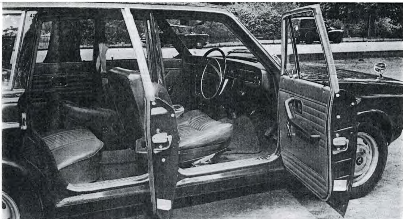
Door openings are generous, making entry and exit easy. Note the carefully contoured front seat and the knob (visible on the far backrest) for adjusting lumbar support
