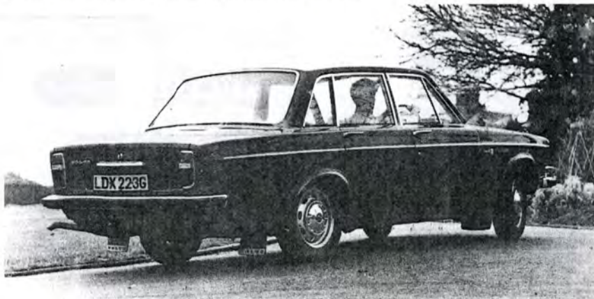
Left: The boot is deep and long, but luggage has to be lifted over a high sill, topped by a rubber strip. Spare wheel and jack are held in with a rubber strap. Below: Practical features include anodized aluminium bumpers with rubber insets, and mud flaps behind each wheel arch
