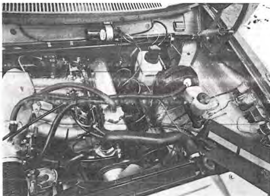
Despite somewhat cluttered appearance, underbonnet accessibility presents no problems. Note cross-over mechanism between brake pedal and direct-acting servo. Same high standard of finish is evident here as elsewhere
