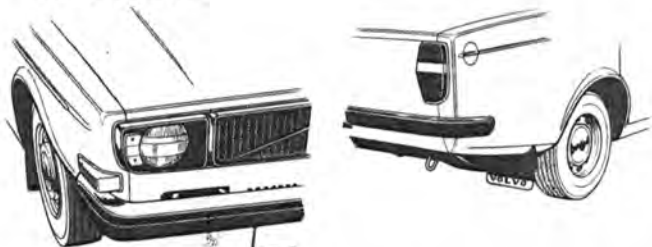
Left: Rubber insert bumpers with chrome decorative strips. Right: Sturdy rear towing loop on right-hand side member. At the front there is another loop on the front suspension sub-frame
