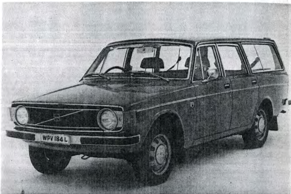
This revised radiator grille, and heavy side-mounted indicator lamps, feature on the Volvo 144 models for 1973. Bumpers are in anodised aluminium
