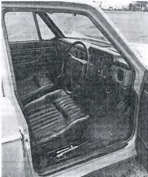
Although reduced in diameter, the steering wheel remains fairly high and close to the driver. Fitted rubber mats are an optional extra
