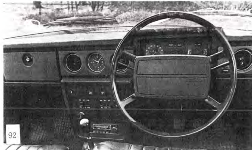
Whole of fascia was redesigned for 1973 model-year. Revised heating/ventilating system features four face-level vents. Note provision for extra switches on centre console
