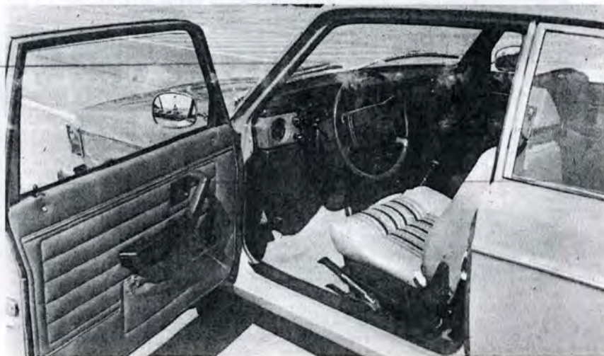
Below: Flame resistant cloth upholstery is now used for the seats, except in the 144GL and 164E, which still have leather. Deletion of the front quarter vents improves visibility and reduces wind noise. The window frames are welded to the doors for additional strength.
