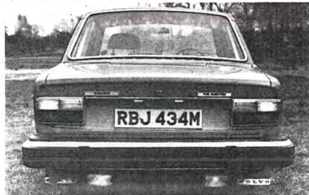
Top: Door handles are recessed, and a rubbing strip protects the sides Above: Huge energy-absorbing bumpers with rubber facings add greatly to the length but afford generous protection Below: Reversing lamps are standard. The test car also had the optional fog rear lamps, mounted beneath the bumper
