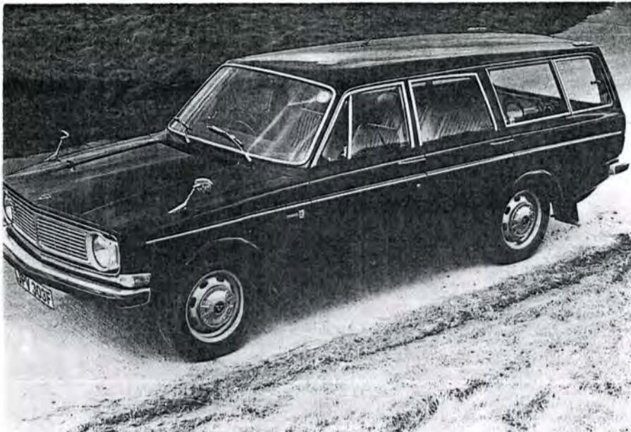
The "extra" window at each side readily identifies the new Volvo. Other features include the rear-wing mounting for the spare wheel, under-floor locker, and rear seat release which can be operated from either side.
