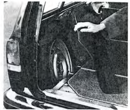
The "extra" window at each side readily identifies the new Volvo. Other features include the rear-wing mounting for the spare wheel, under-floor locker, and rear seat release which can be operated from either side.
