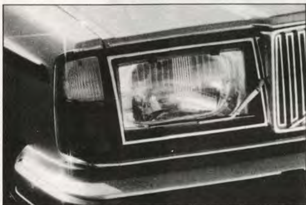
Big rectangular lights with wipers on the 264 aren't likely for the U.S.
